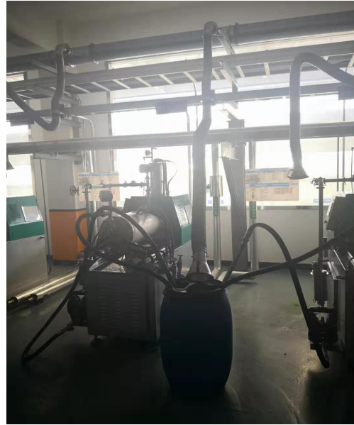
研磨工序集气罩
